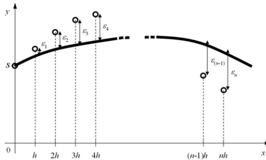
**Fig. 4.** A schematic diagram illustrating differences between the analytical solution  $y(x)$  (the thick solid line) and the approximate computational solution (represented by circles) for the first  $n$  steps after initial conditions  $y(0) = s; y'_x(0) = t$ .
