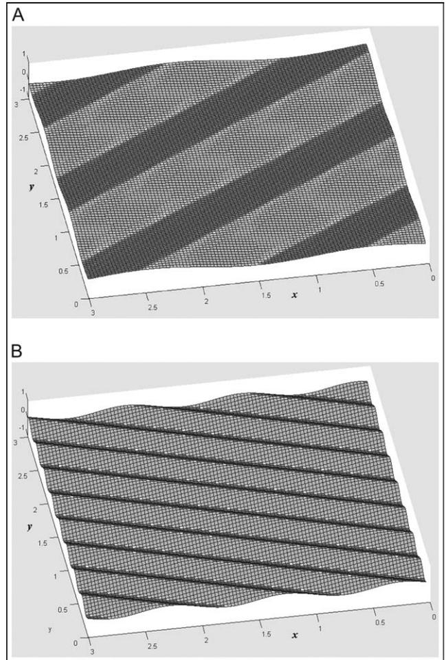
Fig. 3: Numerical simulations of forward scan at  $L = 3 \mu\text{m}$ ,  $v = 3 \mu\text{m/s}$ ,  $A = 0.2 \mu\text{m}$ ,  $d = 0.03 \mu\text{m}$ ; (a)  $\omega = 9.5$  Hz; (b)  $\omega = 18.6$  Hz
