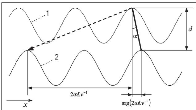
Fig. 2: The observed shift between scanning lines: 1, the first line; 2, the second line of the forward scan
