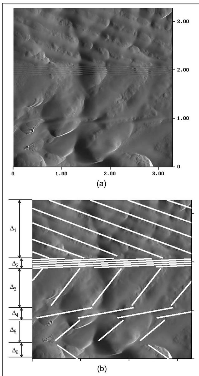
**Fig. 7: Digital image of the scanned surface at varying frequencies of excitation: (a) experimental image; (b) marked white grating lines on top of the image**
