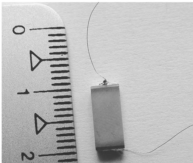
**Fig. 5: Piezoelectric ceramics with welded electrode wires**
