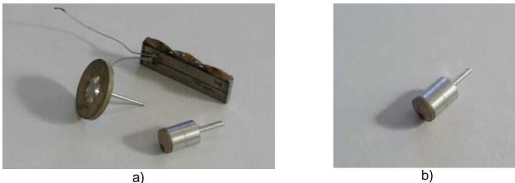
Figure 1. Piezoelectric optical scanners: a- general view of different types of piezoelectric optical scanners developed at Kaunas University of Technology; b- optical scanner with piezoceramic cylinder.
